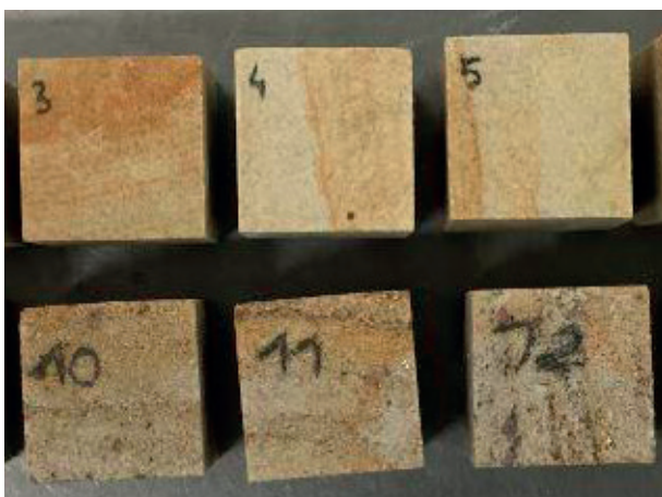
Photo 57. Investigation of the water absorption of sandstone at atmospheric pressure. A view of samples after testing.
