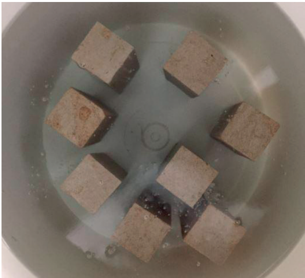
Photo 67. Frost resistance test. Soaking of sandstone samples.
