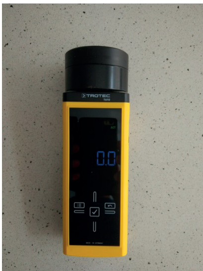
Photo 17. The TROTEC T610 hygrometer
