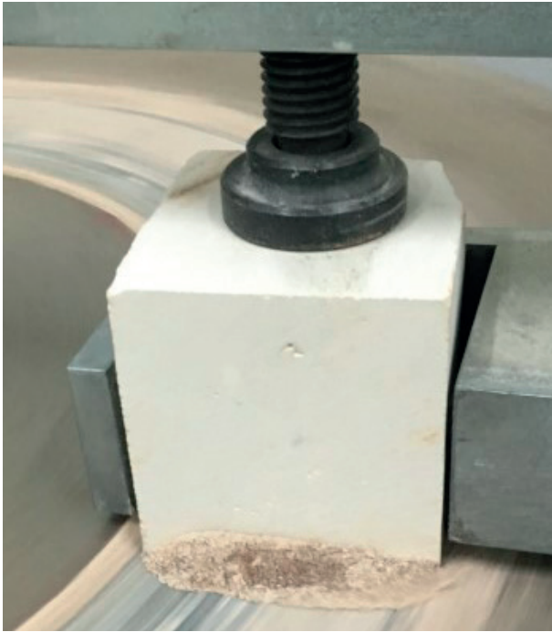
Photo 53. A sample during the abrasion process.
