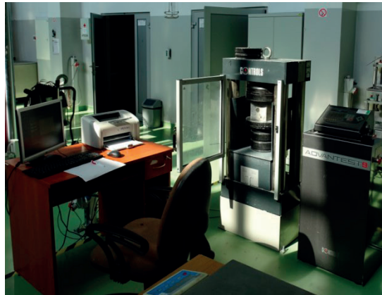
Photo 43. Test station - the Controls Advantest 9 hydraulic press
