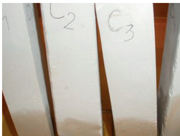
Photo 60. Determination of the capillary absorption coefficient for limestone rock. The end of the study.
