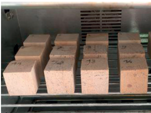
Photo 55. Investigation of water absorption of sandstone at atmospheric pressure. Drying of samples.
