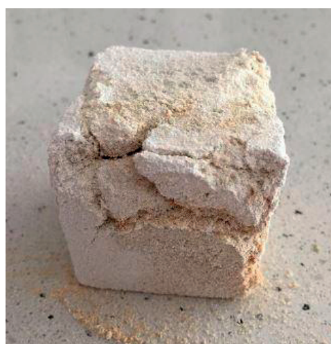
Photo 64. Resistance test for salt crystallization. Limestone rock samples after 10 cycles.
