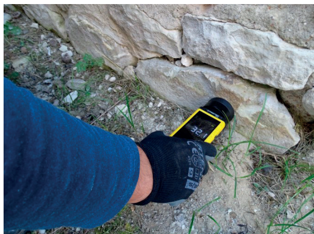
Photo 18. Moisture measurement by the microwave method
