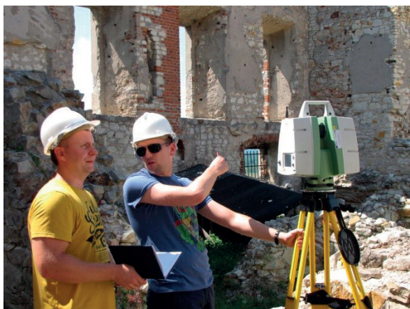
Photo 4. Leica ScanStation C10 while taking measurements
