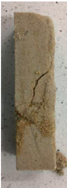
Photo 69. Frost resistance test. A sandstone sample after 30 freezing cycles. 4th degree damage
