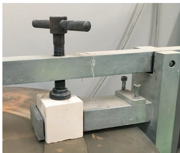
Photo 52. A stone sample mounted in the device holder.
