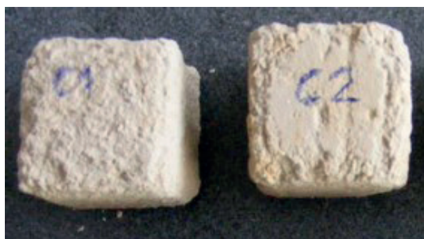
Photo 63. Resistance test for salt crystallization. Limestone rock samples after 2 cycles.
