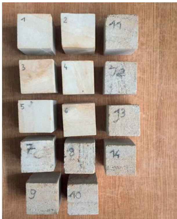
Photo 44. Sandstone samples prepared for compressive strength testing.
