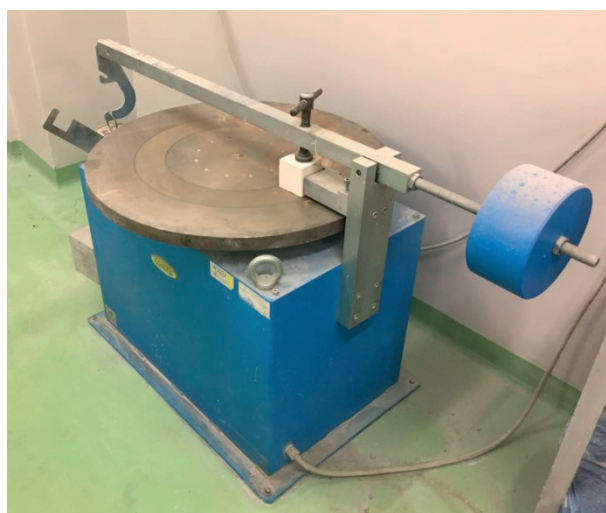
Photo 51. Abrasion testing device - the Boehme's disk.
