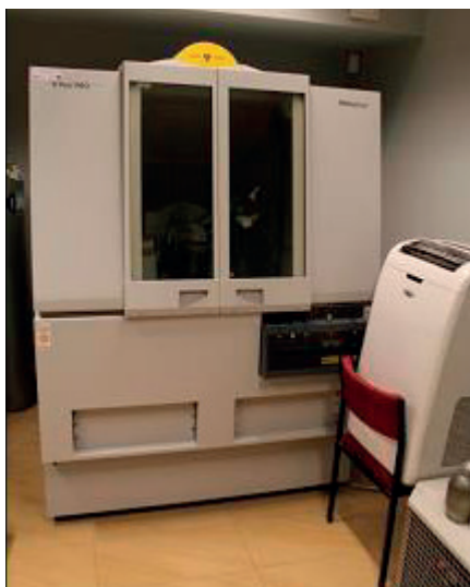
Photo 78. The X-ray diffractometer - X'pert PRO MPD by Panalytical. WBiA laboratory of Lublin University of Technology The XRD measurements of historical materials are made on powdered samples, the mass of sam-
