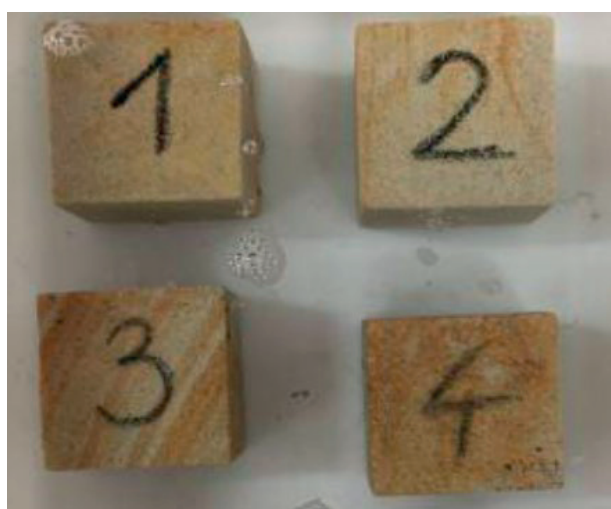
Photo 63. Resistance test for salt crystallization. Limestone rock samples after 2 cycles.
