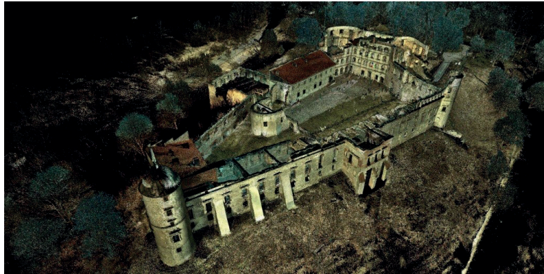
Figure 3. The cloud of points, which was created as a result of the preparation of spatial data obtained from the Leica C10 scanner - Janowiec castle
