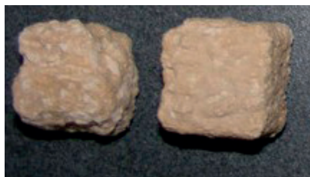
Photo 64. Resistance test for salt crystallization. Limestone rock samples after 10 cycles.
