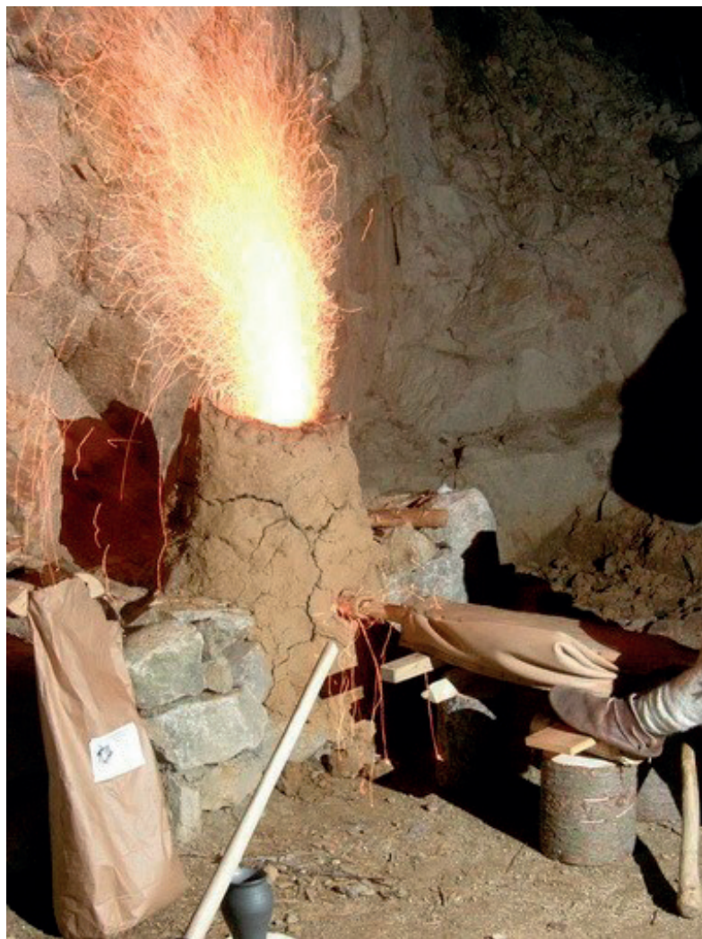
Fig. 22. Pořešín Castle, experimental casting of iron
